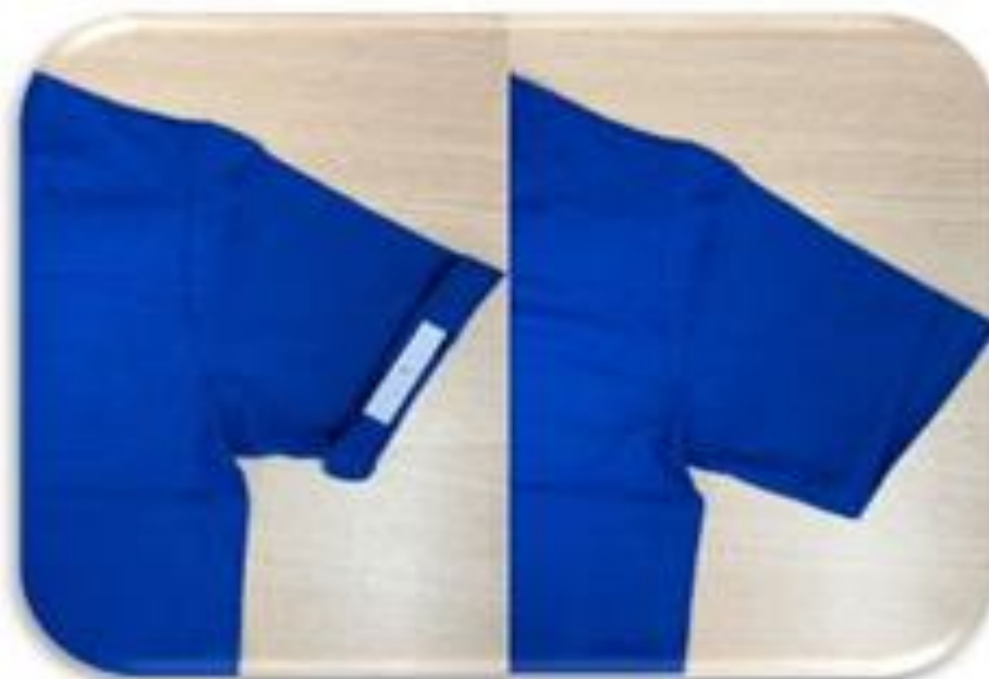
Small and water proof RFID tag/s sewn into the seams of residents' clothes
